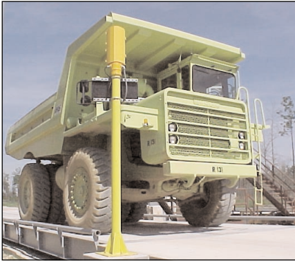
The side-by-side Rodan RC Megabar Truck Scale is capable of weighing heavy off-road vehicles like the Euclid R40, shown above.
