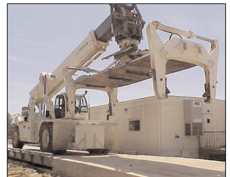
The side-by-side Rodan RC Field Pour truck scale is capable of weighing heavy, off-road vehicles like the TEREX 3308.
