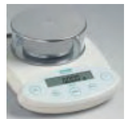
Round draft shield included with mg models
